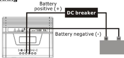
**Step 1:** connect battery positive (+) wire to the positive terminal of the unit and load negative (-) wire to the negative terminal of the unit.
