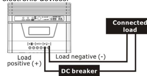
**Step 1:** connect load positive (+) wire to the positive terminal of the unit and load negative (-) wire to the negative terminal of the unit.
